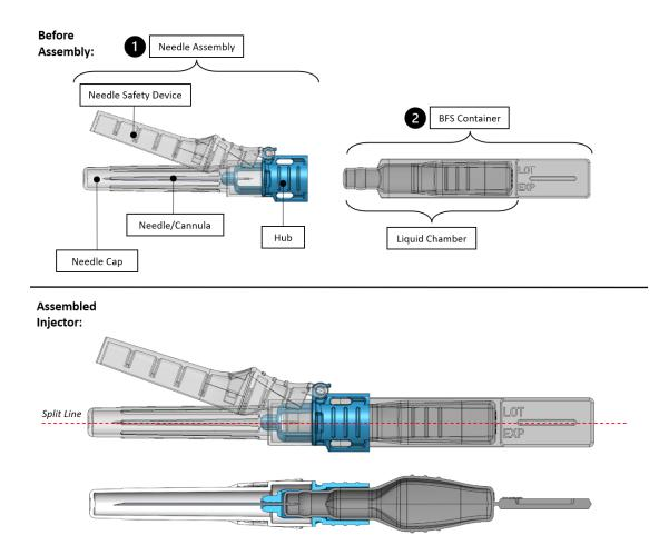
*Figure 1.* Reference Image of an example of a Prefilled ApiJect Injector design (Note: Prefilled ApiJect Injector and Needle Hub have not been cleared by regulators).
