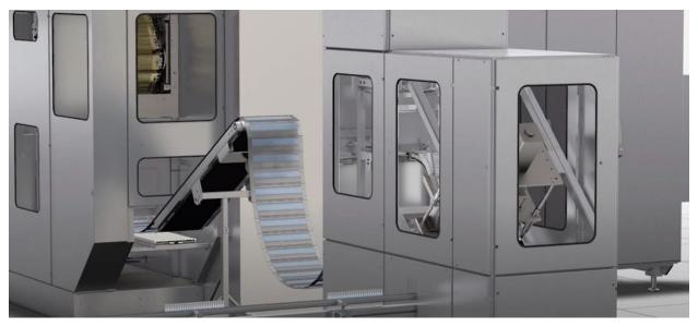
Figure 3. BFS ribbon discharge of BFS machine entering punching station
