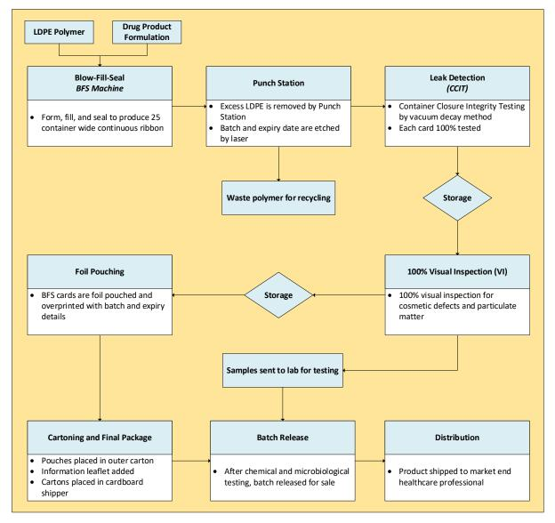
Figure 2. BFS Manufacturing Process Flow Map.
