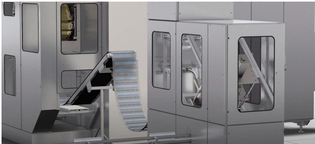
**Figure 3.** BFS ribbon discharge of BFS machine entering punching station
