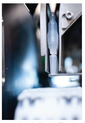
create a ready-to-use drug delivery device. This attachment causes the needle to pierce the BFS container, activating the device. The liquid drug product can then be expelled by squeezing the BFS container. Its simple-to-use injection system is designed to make it a user-friendly product for both healthcare professionals and patients, where allowed by regulators.
