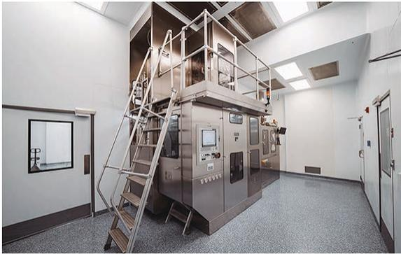
In traditional aseptic (assuming glass vials), the containers are made in one factory, packaged, shipped to a fill-finish facility, unpackaged, cleaned, sterilized, depyrogenated, filled, capped, and then over-capped. Prefilled syringe filling is an equally complex process.
