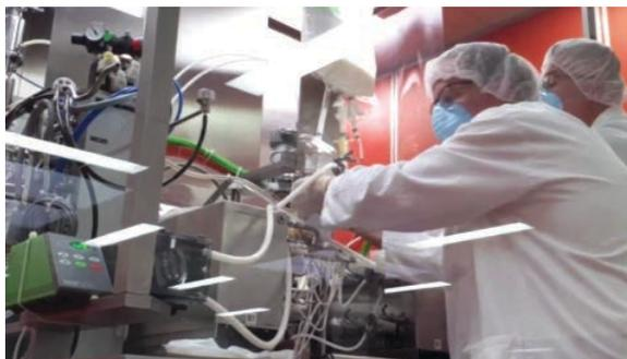
The speed and productivity of high-end rotary BFS machines can be measured in a couple of ways. The entire process of blowing a container, filling it and sealing it can be done in 3 to 7 seconds by a rotary machine, compared to a 10-15 second process for a shuttle machine. Because of this high speed, a single rotary machine can produce up to 25,000-unit dose containers per hour with high “up time” adding to the productivity.
