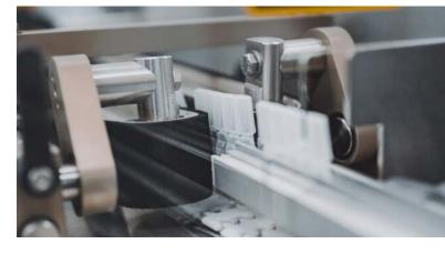
With Blow-Fill-Seal, by creating "just enough" heat, you can produce 25,000 of these plastic containers per hour, aseptically fill them with anything from vaccines to eyedrops, and then seal them, all in strips of 25 at a time, in about 3 seconds per cycle.
